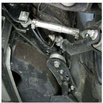
Press in the main bushing from the bottom of the subframe with a shop press. You can use a lubricant like grease or anti seize to minimize binding while pressing in the bushings. Reinstall subframe with the factory retaining plate/washers (pictured) and hardware plus desired shims (see below) and torque the 4 main subframe bolts to 107 ft/lb with a 19mm socket.
